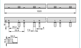
EBU10-Tx2 16 mm<sup>2</sup> 80 A/250 V AC (2-pole devices)
